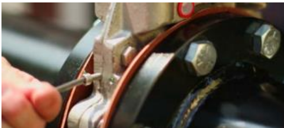
Step 4: Re-install the two packing screws only about halfway into packing holes. This leaves space for future adjustments.
