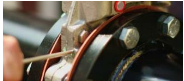
Step 3: Use the packing tool to push each of the two pellets into the packing chamber as far as they will go. Continue to pack one pellet at a time and alternate between holes to ensure even packing distribution.
